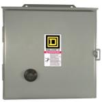
NEMA Starter, Type S, reversing, horizontal, Size 0, 18A, 2 HP at 230 VAC, 5 kA SSCR, 1 phase, 2 pole, melting alloy overload, 208 VAC coil, NEMA 12
