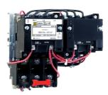
NEMA Starter, Type S, reversing, horizontal, Size 00, 9A, 2 HP at 575 VAC, 5 kA SCCR, 3 phase, 3 pole, melting alloy overload, 24 VAC coil, open
