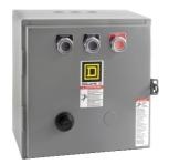
NEMA Starter, Type S, reversing, horizontal, Size 00, 9A, 2 HP at 575 VAC, up to 100 kA SCCR, 3 phase, 3 pole, Motor Logic SSOLR, 208 VAC coil, NEMA 1
