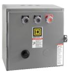
NEMA Starter, Type S, reversing, horizontal, Size 00, 9A, 1 HP at 230 VAC, 5 kA SSCR, 1 phase, 2 pole, melting alloy overload, 120 VAC coil, NEMA 1
