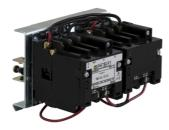
NEMA Contactor, Type S, reversing, vertical, Size 1, 27A, 3 HP at 230 VAC, single phase, up to 100 kA, 3 pole, 120 VAC coil, open style
