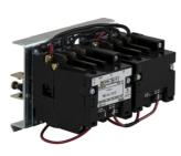
NEMA Contactor, Type S, reversing, vertical, Size 0, 18A, 2 HP at 230 VAC, single phase, 3 pole, 120 VAC coil, open style
