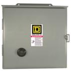
NEMA Contactor, Type S, reversing, horizontal, Size 0, 18A, 5 HP at 575 VAC, 3 phase, up to 100 kA, 3 pole, 24 VAC coil, NEMA 3R/12
