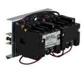
NEMA Contactor, Type S, reversing, horizontal, Size 00, 9A, 2 HP at 575 VAC, 3 phase, 3 pole, 480 VAC coil, open style
