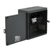
NEMA Contactor, Type S, reversing, horizontal, Size 00, 9A, 2 HP at 550 VAC, 3 phase, 3 pole, 120 VAC coil, NEMA 1
