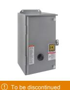
NEMA Motor Starter, Type S, nonreversing, Size 2, 45A, 25 HP at 460 VAC, 5 kA SCCR, 3 phase, 3 pole, melting alloy, 120 VAC coil, NEMA 12
