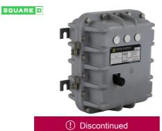
NEMA Motor Starter, Type S, nonreversing, Size 1, 27A, 10 HP at 460 VAC, 3 phase, 3 pole, melting alloy, 120 VAC coil, NEMA 7/9
