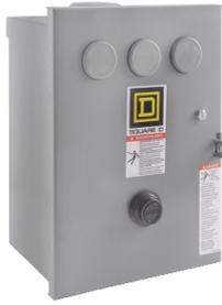
NEMA Motor Starter, Type S, nonreversing, Size 1, 27A, 10 HP at 460 VAC, 5 kA SCCR, 3 phase, 3 pole, melting alloy, 208 VAC coil, NEMA 3R
