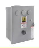
NEMA Motor Starter, Type S, nonreversing, Size 1, 27A, 3 HP at 230 VAC, 5 kA SCCR, 1 phase, 2 pole, melting alloy, 240 VAC coil, NEMA 3R
