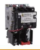
NEMA Motor Starter, Type S, nonreversing, Size 00, 9A, 1 HP at 230 VAC, 5 kA SCCR, 1 phase, 2 pole, melting alloy, 120 VAC coil, open
