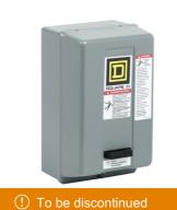
NEMA Motor Starter, Type S, nonreversing, Size 00, 9A, 1 HP at 230 VAC, 5 kA SCCR, 1 phase, 2 pole, melting alloy, 208 VAC coil, NEMA 1
