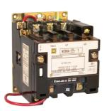
NEMA Contactor, Type S, nonreversing, Size 1, 27A, 10 HP at 575 VAC, 3 phase, up to 100 kA, 4 pole, 120 VAC coil, open
