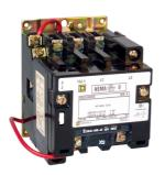
NEMA Contactor, Type S, nonreversing, Size 0, 18A, 5 HP at 575 VAC, 3 phase, up to 100 kA, 3 pole, 600 VAC coil, open
