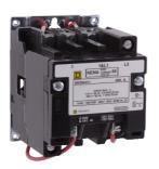
NEMA Contactor, Type S, nonreversing, Size 00, 9A, 1 HP at 230 VAC, 1 phase, up to 100 kA, 2 pole, 208 VAC coil, open
