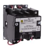
NEMA Contactor, Type S, nonreversing, Size 00, 9A, 1 HP at 230 VAC, 1 phase, up to 100 kA, 2 pole, 480 VAC coil, open
