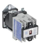
NEMA Control Relay, Type X, utility, 10A resistive at 600 VAC, 4 normally open contacts, 24 VDC coil
