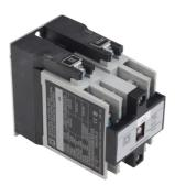
NEMA Control Relay, Type X, master, 10A resistive at 600 VAC, 2 normally open contacts, 110/120 VAC 50/60 Hz coil
