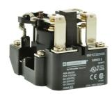
Power Relay, Type C, DPDT, 2 normally open and 2 normally closed contacts, 20A resistive at 110 VDC, 48 VAC coil
