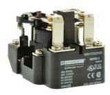
Power Relay, Type C, 20A resistive at 110 VDC, DPDT, 2 normally open and 2 normally closed contact, 208 VAC coil
