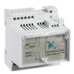
MN delay unit, MasterPact NT/ NW, ComPacT NS, adjustable time delay 0.5s/3s, 100/130VDC, 100/130VAC 50/60Hz, spare part
