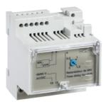
MN delay unit, MasterPact NT/ NW, ComPacT NS, adjustable time delay 0.5s to 3s, 48/60VDC, 48/60VAC 50/60Hz, spare part
