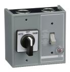
Manual Starter, fractional horsepower, duplex, 16A, 2 poles, 1 HP at 277 VAC, toggle and selector, red indicator, NEMA 1
