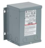
Transformer, buck boost, encapsulated, 1kVA, 1 phase, 240x480V primary, 24/48V secondary, NEMA 3R, 115C rise
