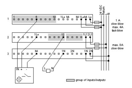
4-Wire Sensor with a 3-Wire Actuator
