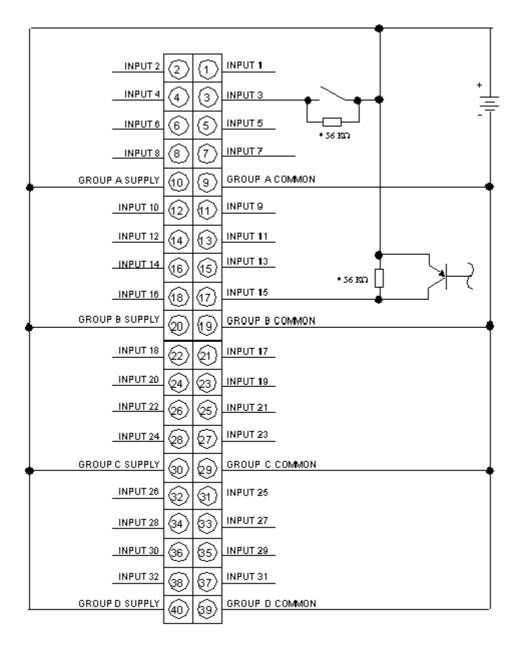
\* Recommended resistor value for 24 Vdc.
