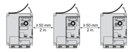
For Operation at Ambient Temperature Above 50  $^{\circ}\text{C}$  (122  $^{\circ}\text{F})$
